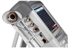
You can connect various accessories like the GPS receiver R&S HA-Z240 (order no. 1309.6700.02) to the AUX connector.
