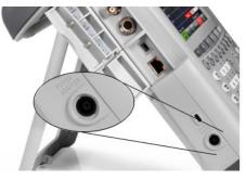
The R&S ZVH is supplied with power by the AC/DC transformer power supply via the DC connector. You can also use the DC connector to charge the battery.
